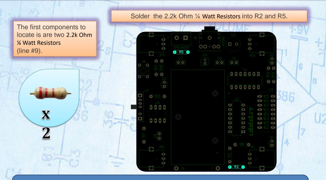
Axial Lead Resistors such as the ones used in this kit are color coded. Compare the resistor you are installing to the images shown in each step. Also double check the values with a multimeter on the ohm setting.
