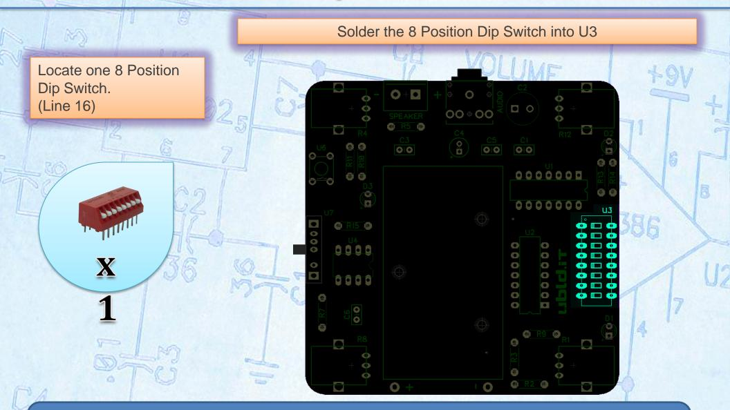
The 8 Position Dip Switch feeds the inputs of the 7-Stage Ripple-Carry Binary Counter (U2).
