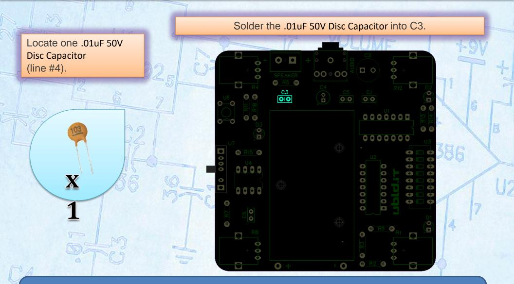
Capacitors store an electrical charge much like your body builds and stores static. It's also good to know that since a capacitor takes time to charge and discharge it's said that it opposes changes in voltage.
