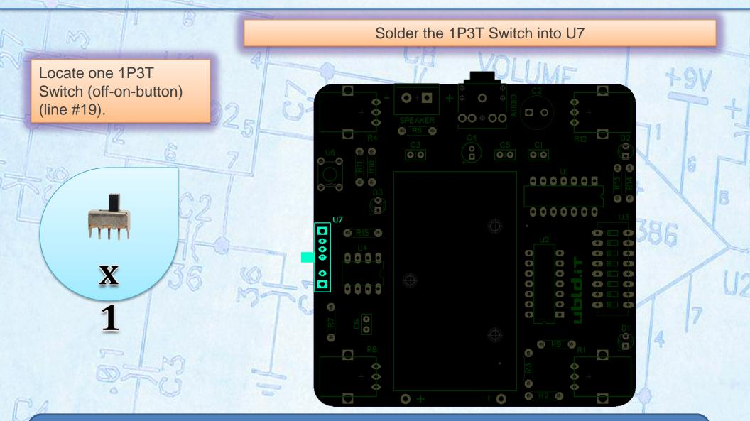
The 1P3T Switch has 3 positions. Off turns the device completely off. On provides continuous audio. And Button provides audio only when the U6 Momentary Switch is pressed.
