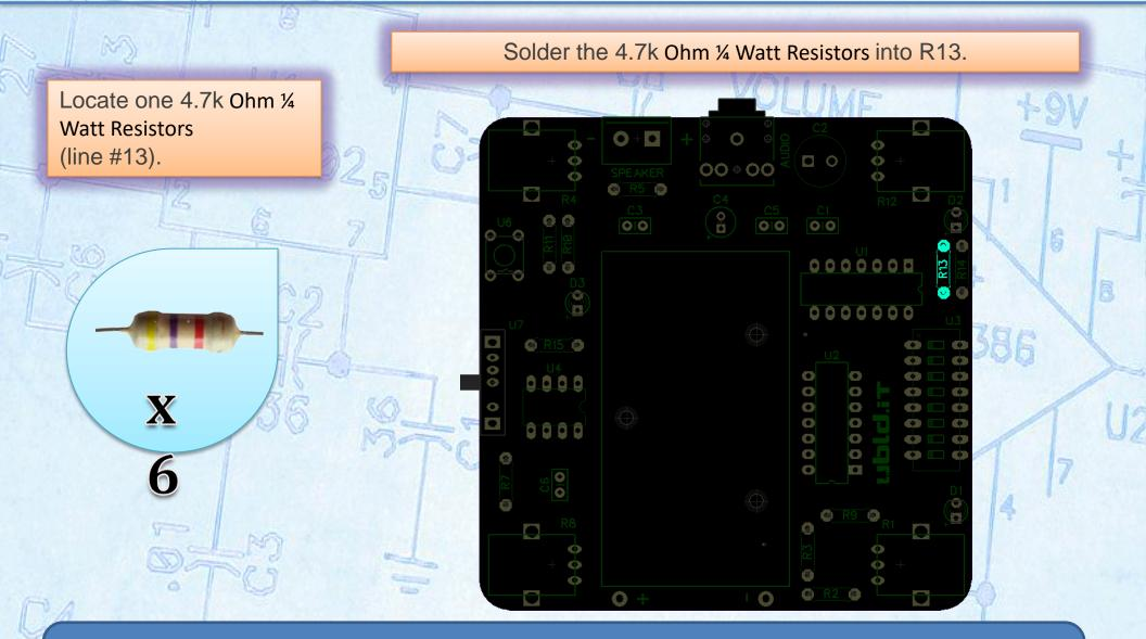
For better looking solder joints use Kester #2331-ZX water soluble flux pen on every pad before applying solder. Flux removes oxidation and allows heat to transfer from your iron to the pad.
