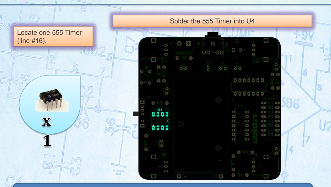
The 555 Timer is a iconic integrated circuit which is used in many beginner electronic circuits. Take some time and do a little homework on this IC.
