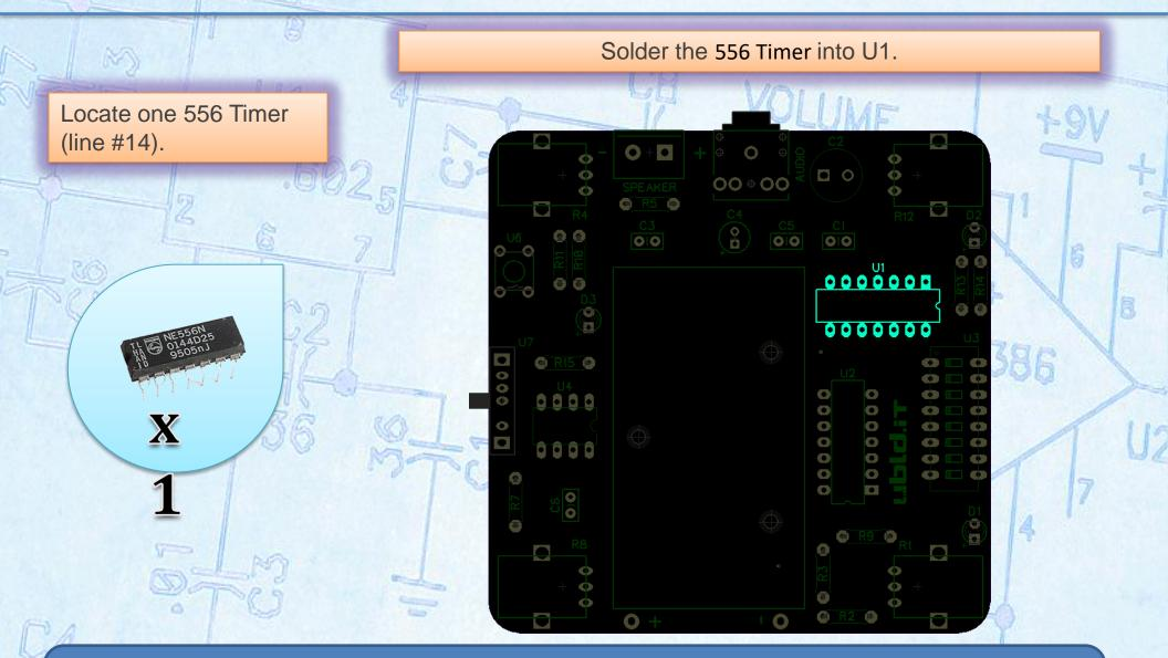
Pin one of the IC is marked with a small indentation in the package. Orient the package indentation with the silkscreen indentation.
