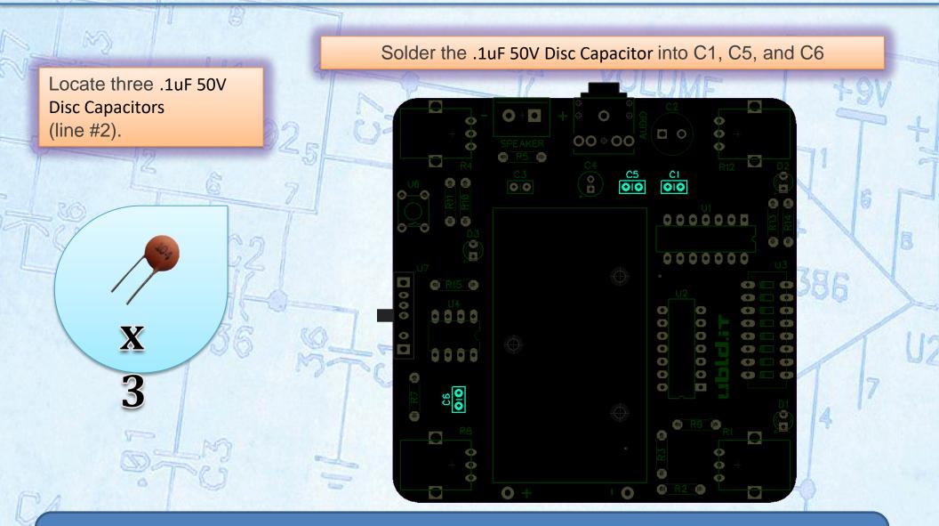
Ceramic capacitors are not polarized so orientation doesn't matter.
