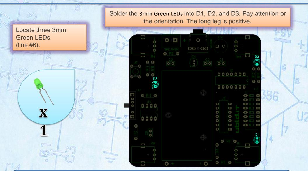
Diodes are polarized. The long leg of this LED is the positive (Anode) and the short leg is negative (Cathode).
