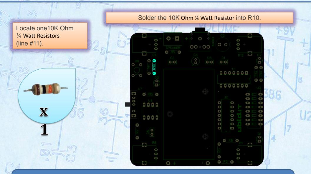
It's not necessary for resistors, but inserting them all in the same direction will make your board look that much better. Use the last band (tolerance band) as a reference for the orientation.
