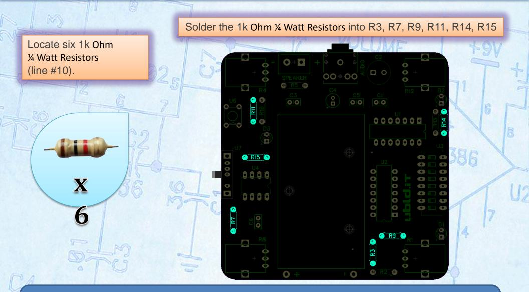
Take pride in your work. Take your time to bend all the components leads to 90 degree angles using needle nose pliers.
