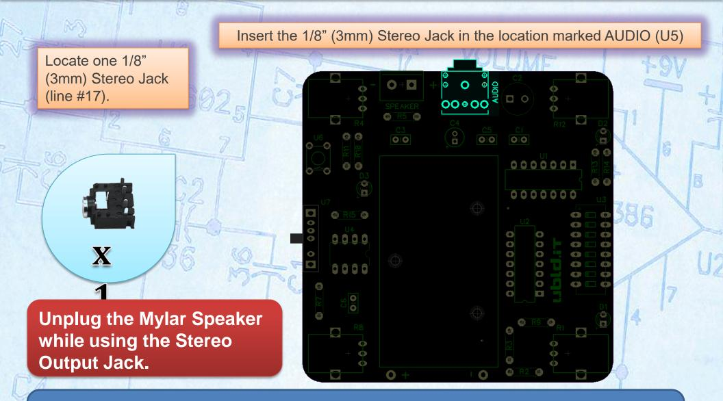
The stereo jack provides an output which can be fed into an Audio Amplifier. You are not limited to using the included Mylar speaker. Disconnect the Mylar speaker when using the AUDIO stereo out jack.
