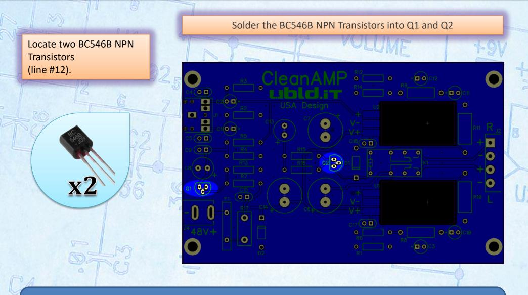
Transistors are used for signal amplification and switching. In the case of the CleanAMP it's used as a switch to enable the K1 relay.
