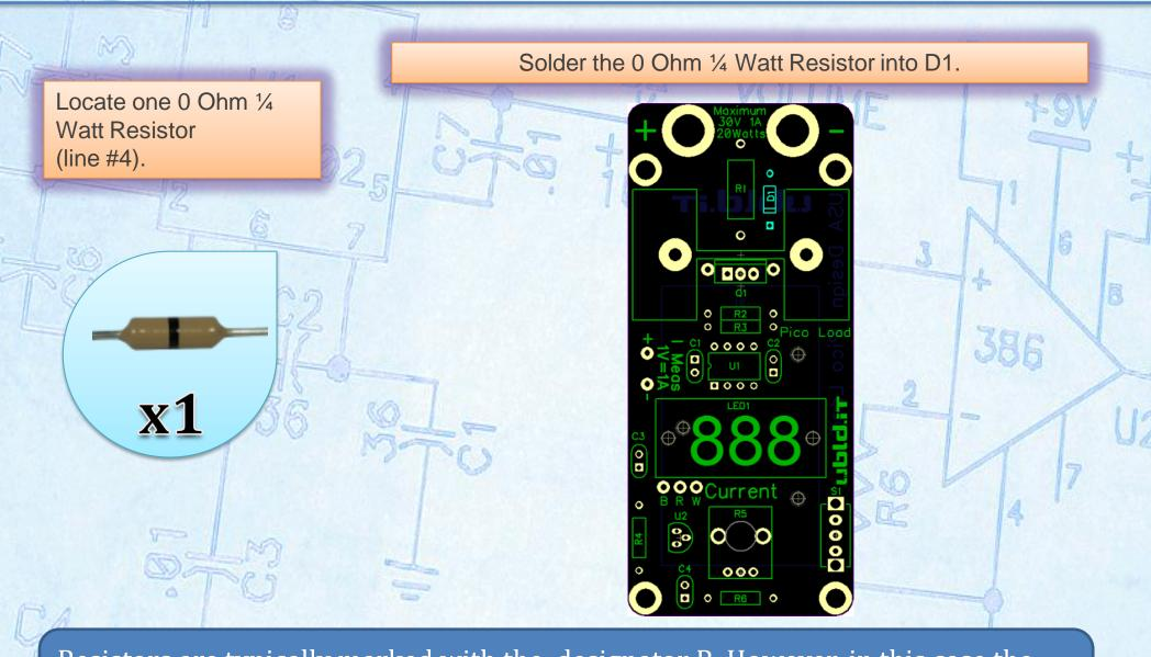
Resistors are typically marked with the designator R. However, in this case the original diode was replaced with a 0 Ohm Resistor. This part substitution is just one of a few which has allowed us to increase current rating on the Pico Load.
