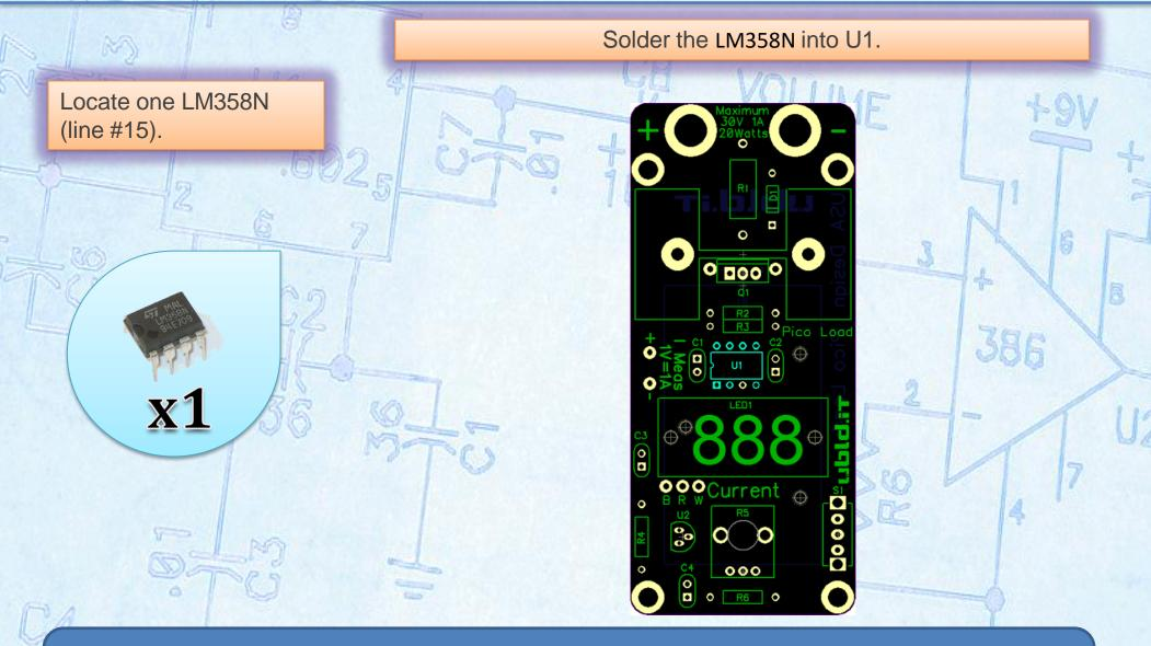
Pin one of the IC is marked with a small indentation in the package. Orient the package indentation with the silkscreen indentation.
