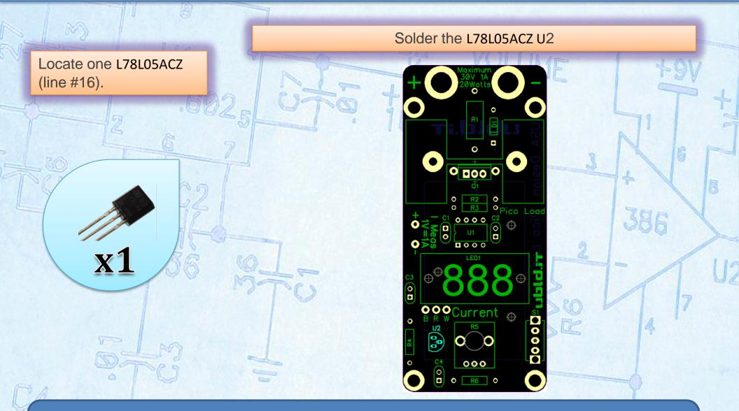
U2 is a 5V Regulator in a TO-92 package. This small package also has current limiting and thermal protection making virtually indestructible.
