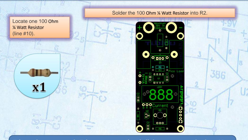
Take pride in your work. Take your time to bend all the components leads to 90 degree angles using needle nose pliers.
