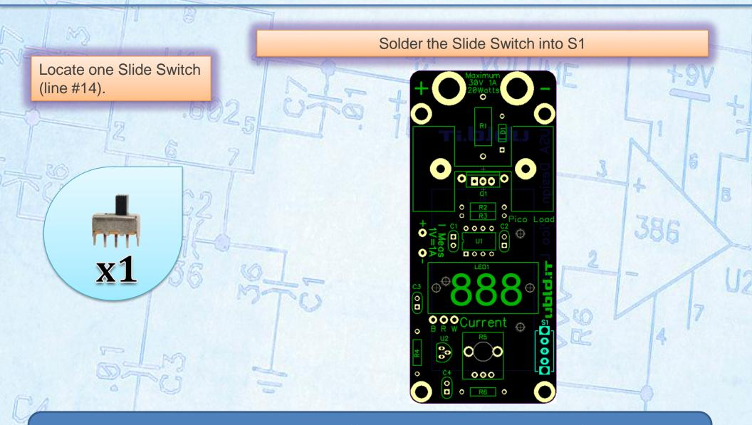
SW is used to turn the circuit on and off. It's a good idea to turn R5 full counter clockwise (down) before turning power on.
