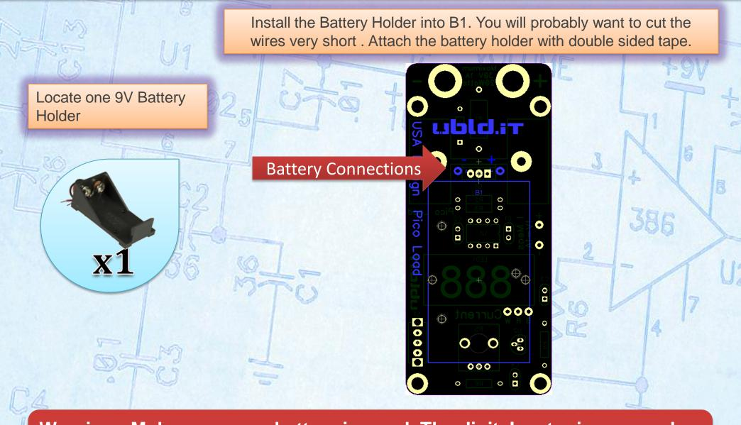
Warning: Make sure your battery is good. The digital meter is powered directly from the 9V battery and low voltage will throw off the readings.
