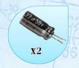
Solder the 22uF 50V Electrolytic Capacitors into C3 and C12.
