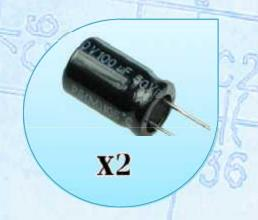
Solder the 100uF 50V Electrolytic Capacitors into C8 and C13.
