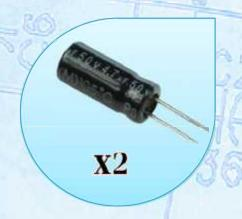
Solder 4.7uF 50V Electrolytic Capacitor into C1 and C2.
