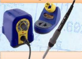
We recommend the Hakko FX888 or similar iron with a chisel tip.
