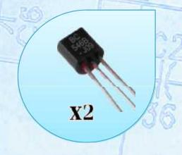
Solder the BC546B NPN Transistors into Q1 and Q2
