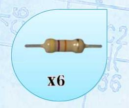
Solder the 47k Ohm ¼ Watt Resistors into R4, R5, R6, R7, R14 and R15.
