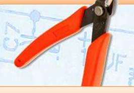
Small cutters for clipping excess wire leads after soldering.
