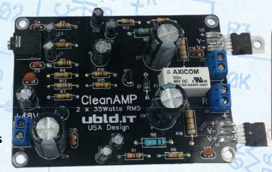
Don't forget to mount the TDA2050 Amplifiers to a Heatsink.
