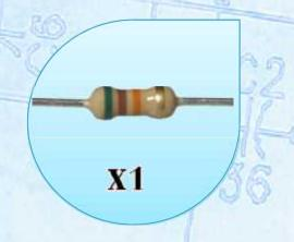
Solder the 51K Ohm ¼ Watt Resistor into R13.
