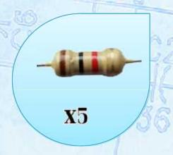
Solder 1K Ohm ¼ Watt Resistor into R1, R2, R3, R12 and R16.
