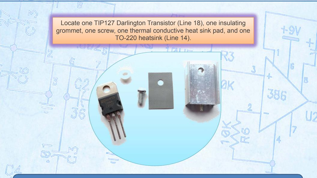
The insulating grommet and thermal conductive heat sink pad are considered to be part of the TO-220 heatsink from line 14.
