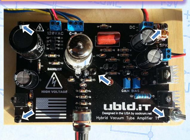
Inserting the center screw first will allow you to easily reposition the corner standoffs should they become misaligned.
