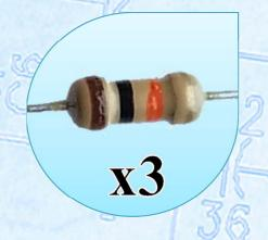
Solder the  $10k\Omega \frac{1}{4}$  Watt resistors into R7, R12 and R15.
