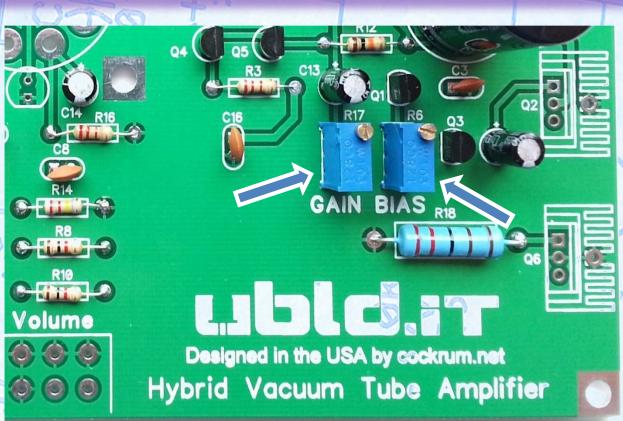
Solder the 10k Ohm Potentiometers into R6 and R17. Warning!
