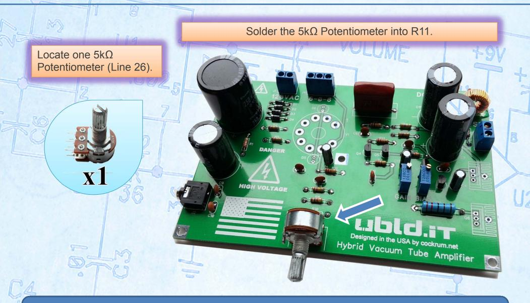
R11 controls the audio volume. It is used as a voltage divider controlling the input signal level to the tube.
