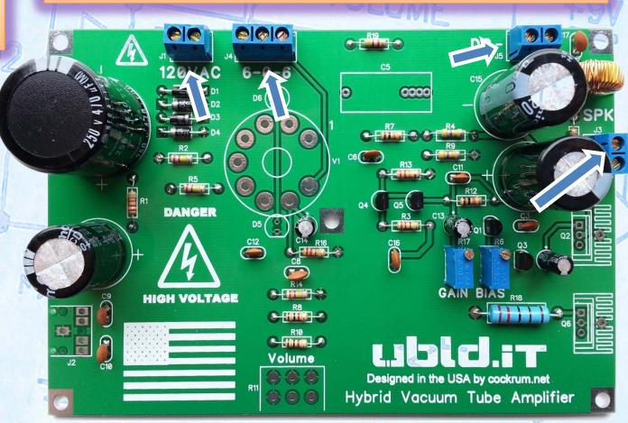
Take the time to align the terminal blocks parallel with the edge of the circuit board. It's possible for them to be aligned a little slanted.
