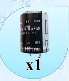
Solder the 470uF Capacitor into C1. **Danger!** This component will explode violently if inserted backwards.
