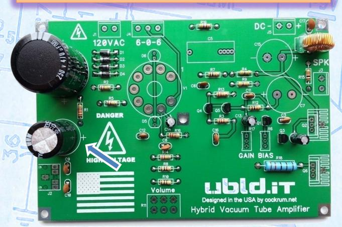
Warning: Inserting any of the polarized capacitors backwards will cause them to explode violently. Double check the polarity for all electrolytic capacitors.
