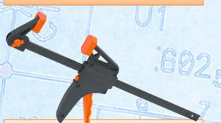
Used for holding parts in place while pre-drilling.
